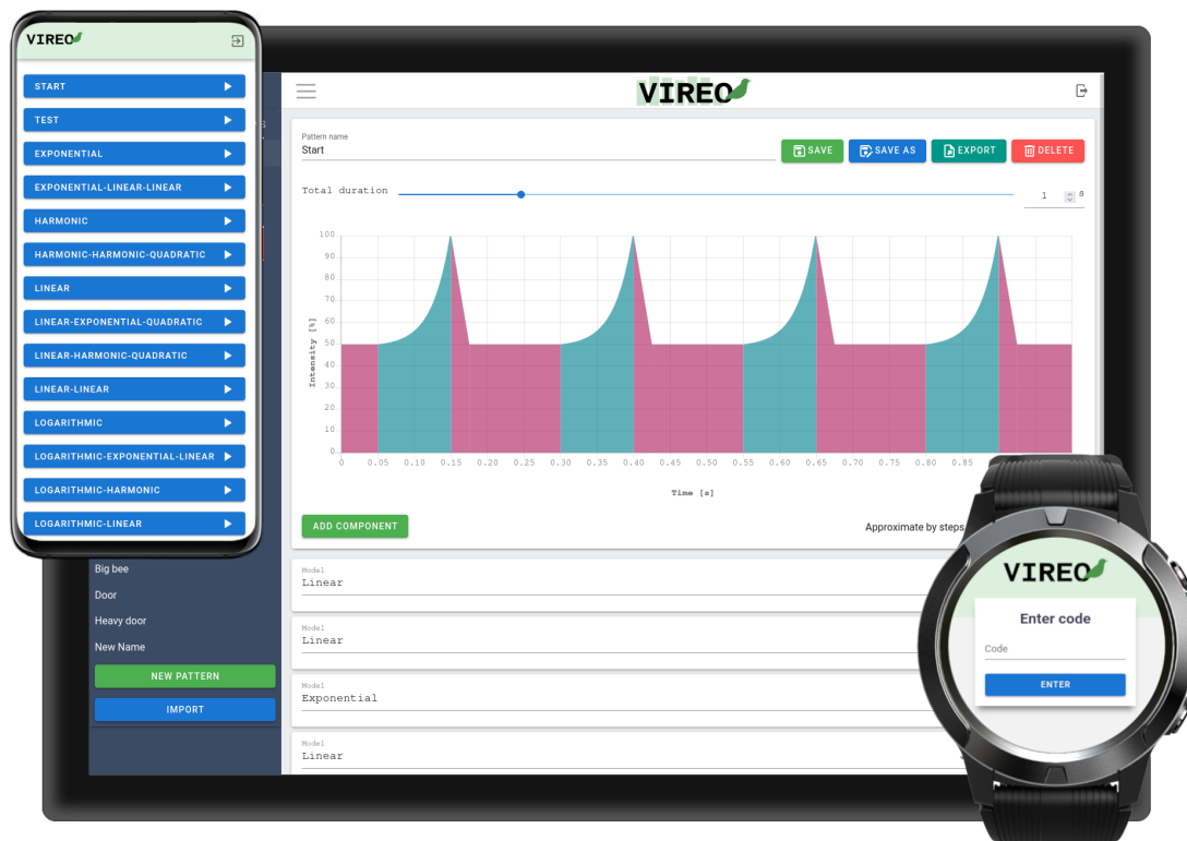
Figure 3.1: The multimodal haptic framework, VIREO [79], freely available at https://vireoapp.com , enables graphical authoring of vibrotactile and audio feedback patterns for augmenting interactions on mobile and wearable devices.
