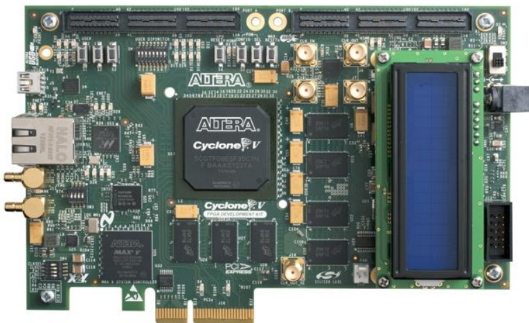
Figura 18 Cyclone V - 5CGTFD9E5F35C7 de la ALTERA
